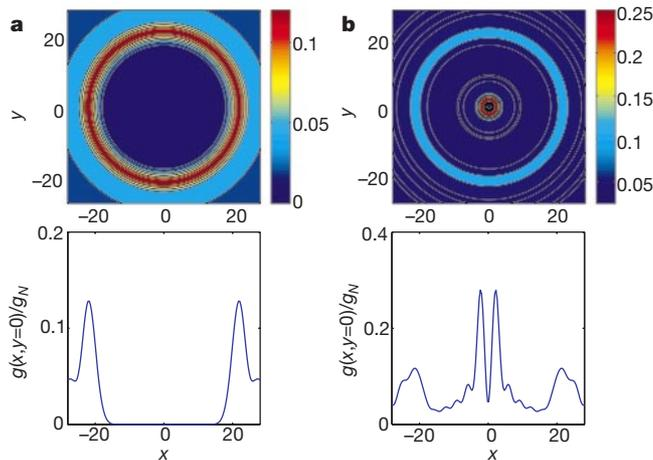
Figure 2 Spatial distribution of the thermodynamically averaged local DOS  $g(\mathbf{r})$  normalized by its normal state value  $g_N$  for multi-quanta vortices. a,  $m = 2$ ; b,  $m = 3$ . The  $x, y$  coordinates are measured in  $1/k_F$ ,  $T \approx \Delta/k_F\xi$ ; for  $m = 2$ ,  $k_F r_c = 20\sqrt{2}$ ; for  $m = 3$ ,  $k_F r_c = 40/\sqrt{3}$ .
