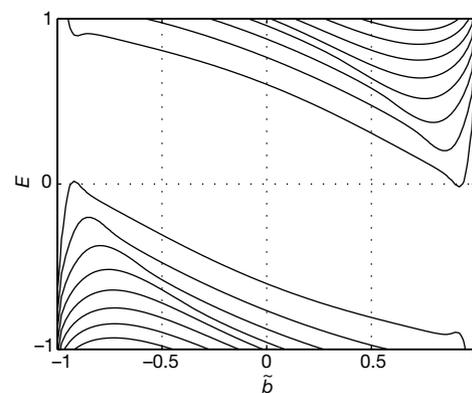
**Figure 4** Energy spectrum for electronic states at the sample edge. Parameters used in these calculations are:  $H = H^* = \phi_0/(\pi R\xi)$ ,  $R = 15\xi$ ,  $|k_\perp|/k_F = 1$  (see text for details).  $\tilde{b} = \mu/(k_\perp|R)$  is the dimensionless impact parameter.
