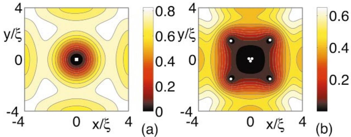
FIG. 4. (Color) Contour plots of the  $|\Psi|$  for (a) double-quantized vortex ( $H=0.65$ ) and (b)  $3\Phi_0$ -molecule situated in the center ( $H=1.26$ ,  $\mathcal{N}=7$ ). The white circles denote singly-quantized vortices, the white square denotes the double-quantized vortex.
