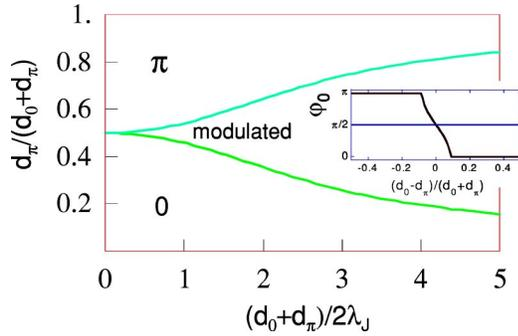
FIG. 1. (Color online) Phase diagram of the periodic alternating  $0-\pi$  junction structure. Inset shows dependence of the equilibrium phase on the length mismatch, for  $d_0 d_\pi = \lambda_J^2$ .
