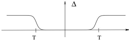
FIG. 2. Dependence of the order parameter  $\Delta$  on time  $\tau$ . The region  $\tau > 0$  is the mirror reflection of the “physical” region  $\tau < 0$ . The superconducting state corresponds to the regions  $|\tau| > T$  while the paramagnetic one to  $|\tau| < T$ .
