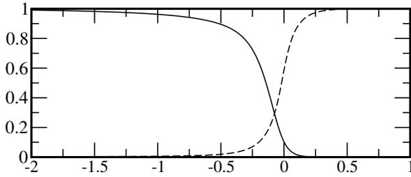
FIG. 3. The normalized order parameter  $\Delta(\tau)/\Delta_0$  (dashed line) and the normalized total spin  $2S(\tau)/N$  of the grain as functions of  $\tau' = \tau - T$  at the boundary  $\tau \sim T$  between the superconducting (left) and paramagnetic (right) states.
