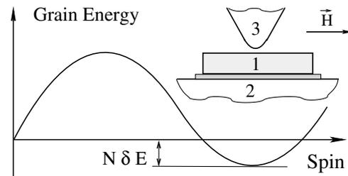
FIG. 1. Energy of an isolated superconducting grain as a function of its total spin. The inset shows a possible experimental setup: An STM tip (3) and superconducting grain separated by an insulating layer from metallic plate (2).
