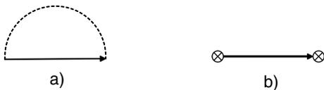
FIG. 3. Diagrams describing self-energy corrections to the single electron propagator due to (a) elastic interaction of electrons with impurities and (b) electron hopping. The solid lines denote the bare propagator of electrons and the dashed line describes the elastic interaction of electrons with impurities. The tunneling vertices are described by the circles.
